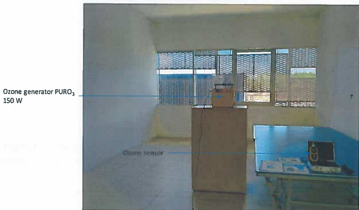
Figure 2. Ubication of the ozone generator (PURO 3 150 W) and ozone sensor in the testing space of 78.7 m 3 .
